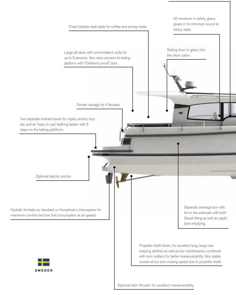
Sliding side-door with access to deep side deck from the helm. Also easy and safe step-off from boat with opening in the pulpits.
