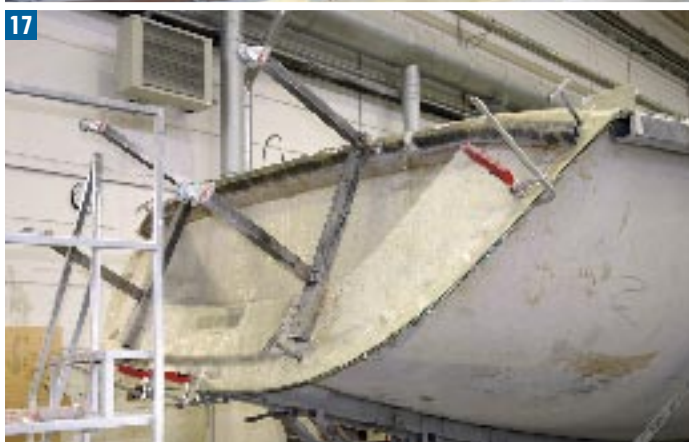
12, 13 & 14 Laminated in and neatly finished, galvanised steel frames reinforce all Grand Soleil hulls, save for the Grand Soleil 56. The first to get the treatment was the four-to-five-year-old Grand Soleil 45. Those frames and their 'wings' resolve chain-plate, mast-step and keel-bolt loads. It is much more efficient structurally than a conventional FRP laminate. All the internal hull surfaces that are visible or could be accessed from inside the boat are painted with this brown gelcoat, which is believed to contrast nicely with the joinery veneers. 15 The deck lamination area: note the MVP resin-mixing equipment. 16, 17, 18 & 19 Transoms are laminated separately. While still in the tool they are clamped into place at the back of the main hull tooling assembly. They are then laminated into place. The resulting joint is very neat and requires minimal dressing. Much of the flash can be broken off between the fingers.
