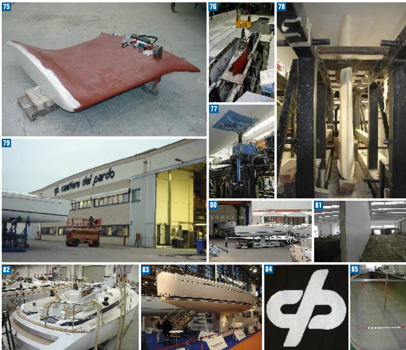
75. 76. 77 & 78 There are two stations on the line for attaching keels. The keels are located using jigs and hulls are leveled to the waterline using jacks at each cradle corner. The keels are aligned with the help of laser-sighting equipment. 79 & 80 The hardstanding at the front of Grand Soleil's Forlì plant: note the outdoor finishing area in the canvas walled and roof building at the end. The main assembly hall on the site will soon be lengthened to provide extra space for this function, so everything will eventually be handled under cover of the main building. 81 A major plant expansion is currently underway. These new halls will be ready for spring 2007. They will accommodate a completely new joinery shop and model-development areas. More land adjoining this site is available for further expansion too. 82 Such is the flexibility of the Grand Soleil line that it can accommodate the odd strange request. Check out this old Grand Soleil 43 model that went down the line in December. It is destined for a customer insistent that he wanted an identical new version of his old boat and not the latest Grand Soleil 43 replacement. Note the old-fashioned rake to transom and the bold strip along the coachroof. 83 The all-new Grand Soleil 40, on display at Paris's Salon Nautique 2006 in December. 84 The Grand Soleil logo represents a 'dp' — which stands for Cantieri del Pardo. 85 The hull of the new Luca Brenta-designed Grand Soleil 53 is soon to move into the fit-out area, although the first one or two will be built off line. A 3D scanner was used to map the precise internal shape of this first hull, the data from which will be used for the interior design process and subsequently the CNC cutting of joinery panels. Six-and-a-half staff are said to be involved permanently with this prototyping work — two handling time and methods, two doing prototyping joinery and two-and-a-half doing deck layouts.
