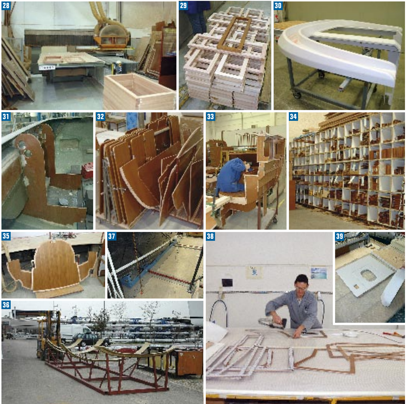
28 & 29 The joinery shop benefits from a number of CNC routers. 30 A sprayhood moulding that includes companionway hatch framing for a Grand Soleil 56. 31 Plywood divides the lazarette of this new Grand Soleil 40, either side of the rudderstock. Note the holes for various wiring and trunking. 32 Bulkheads and doors 'ready to go'. Mahogany is the standard veneer choice throughout the range; teak is optional. 33 As much of the interior as possible is put together in modules that can be craned into position. 34 Wooden-parts store. 35 Note the way the edges of this bulkhead have been stripped bare to provide a key when they are glassed into position. 36 & 37 Hulls are carried down the assembly line on cradles. The line moves under power every 12 hours or so. The forklift truck shunts the empty steel cradles from the end of the line back to the start. There are no wheels on them. They just slide over the concrete — noisy, but efficient. 38 & 39 Most of the upholstery is handled in-house.
