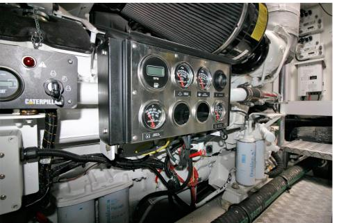
The large and easily accessible engine room. Two Caterpillar C32, 1652 Hp diesel engines, as well as all other technical equipment. (450 engine hours). Last serviced in 2015/16
