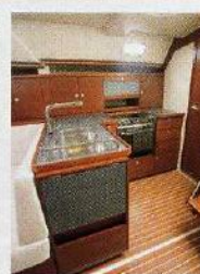
LEFT: The saloon is neat, modern and roomy, with a mahogany fit-out. ABOVE: The 'cafe-style' chart table is inadequate and the galley sinks are rather too shallow for ocean passage-making
