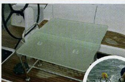
ABOVE: With the plexiglass cockpit table unfolded, four crew can dine in style.
