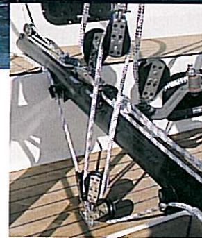
Mainsheet can be finely trimmed with one hand.
