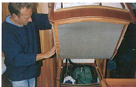
Hinging steps on gas struts make access to the engine simple and comprehensive
