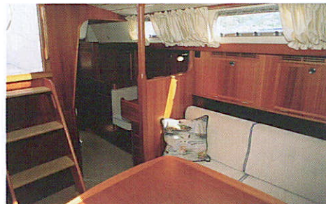
The passage aft uses the full height of the cockpit coamings for headroom
