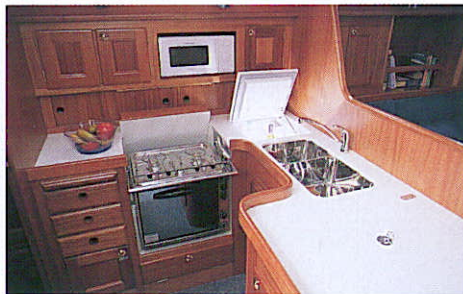
A good worktop space and excellent handholds make the galley safe for sea
