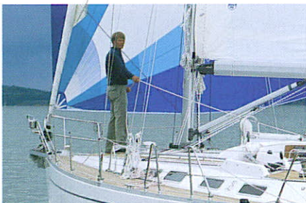
Furler and gennaker fittings forward of the bow roller make sail handling easy
