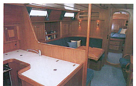
Placing the galley abaft a bulkhead helps split the interior without making it cramped
